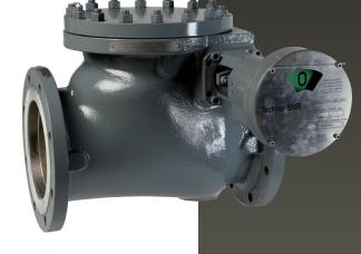
They are based upon swing check valves, designed to secure tanks containing flammable products. They are normally open in tank operation and the action of a rotative system made of fuses and spring will close them automatically when the temperature increases above a preset value, like for example in case of a fire.
